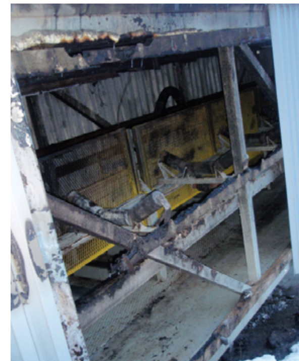
Figure 7: Enclosed conveyor after fire (Source: MVW).
