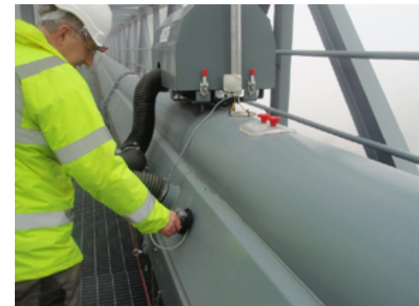
Figure 12: Detail of the "VecoBelt": A fan supplies the required air for the air cushion (Source: MVW).
