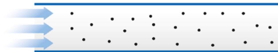
Figure 1: Dispersed flow conveying according to [1], courtesy of Prof. Dr. Ing. habil. Karl-Ernst Wirth, University Erlangen, Germany.
