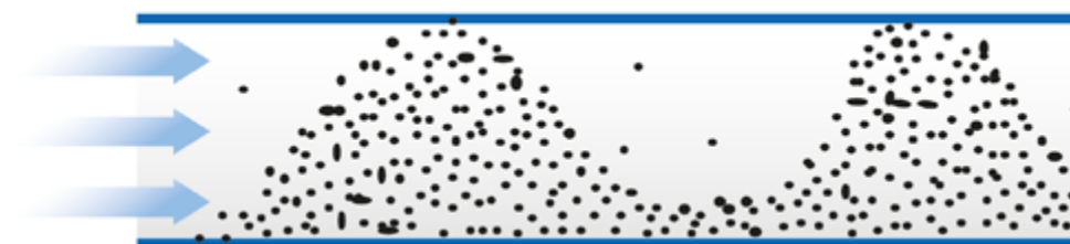
Figure 2: Pulse flow according to [1], courtesy of Prof. Dr.-Ing. habil. Karl-Ernst Wirth, University Erlangen, Germany.
