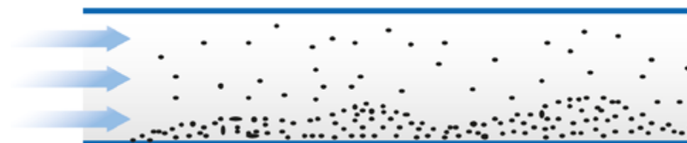
Figure 3: Layer dispersed flow according to [1], courtesy of Prof. Dr.-Ing. habil. Karl-Ernst Wirth, University Erlangen, Germany.
