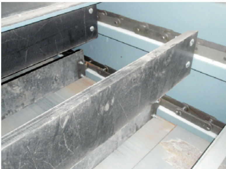
Figure 8: Detail of a drag chain conveyor for alternative fuels with scrapers and chains (Source: MVW).
