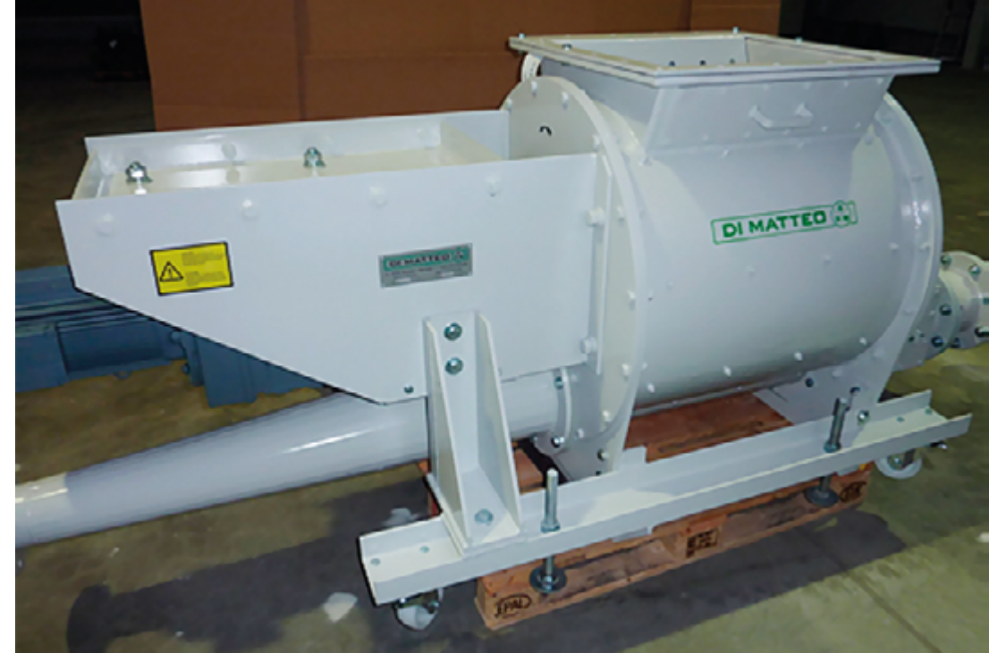
Figure 5: Injector jet with airlock (Source: Di Matteo Fördertechnik, Germany)
