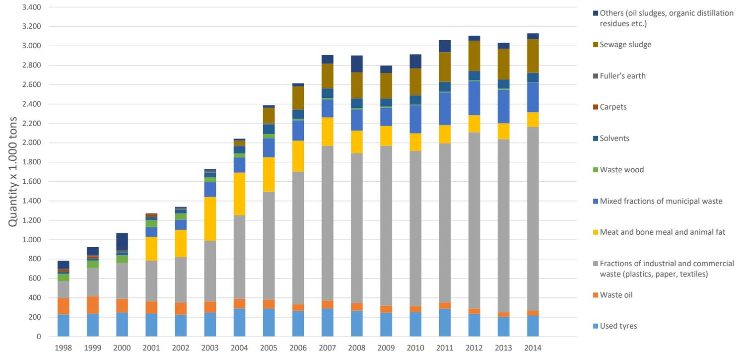
**Figure 5** Presentation of the trend in alternative fuel portfolio in the German cement industry; numbers according to (5).
