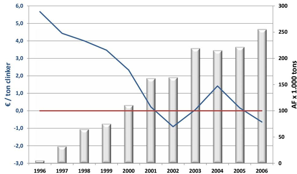
**Figure 7** Trend in entire specific fuel costs (left axis) and utilisation of different kinds of alternative fuels, displayed as summarised columns (right axis) (source: MVW).
