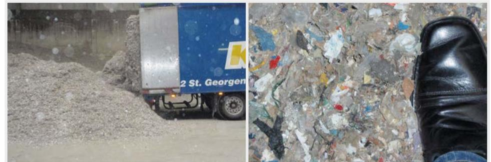
**Picture 1** Unloading “fluff” from a Walking-Floor® truck into the storage hall of a cement plant for kiln burner feeding (left); close-up of the fluff (right) (source: MVW).
