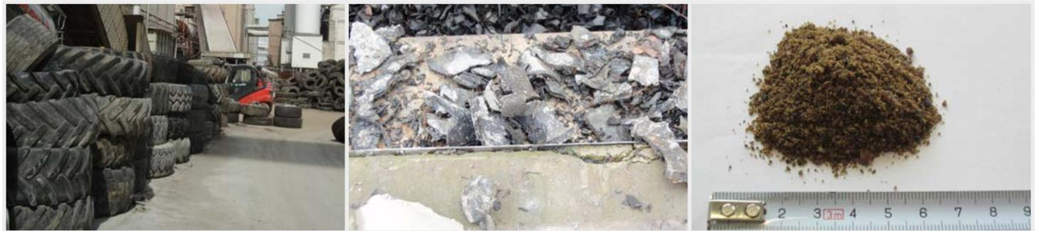
**Picture 2** Storage of whole tyres for kiln inlet feeding (left); tyre chips for kiln inlet feeding (centre); animal meal for kiln burner firing (right) (source: MVW).
