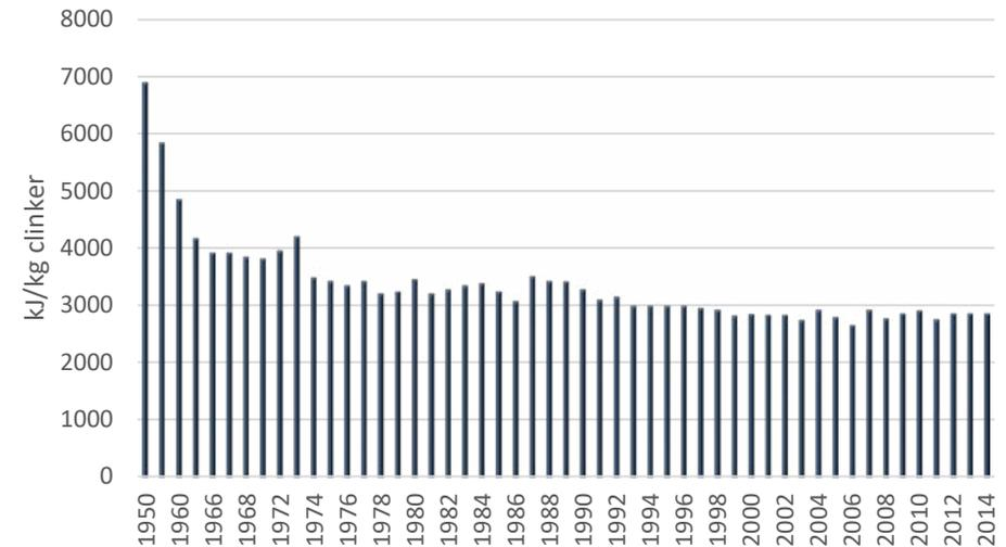
**Figure 2** Trend in specific thermal energy consumption, expressed as kJ/kg clinker; numbers up to 1987 reflect only Western Germany, the following years cover entire Germany; numbers according to (4).
