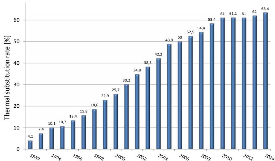
**Figure 3** Average utilisation of alternative fuels in the German cement industry in terms of thermal substitution rate; numbers according to (5)
