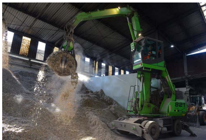
Figure 2: The loading or conveying process produces a substantial amount of dust and places high technical demands on fire detection.
