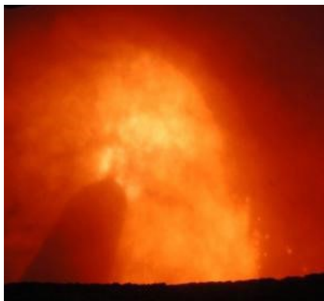
Figure 3: The typical kiln burner flame of highly luminous reddish-orange colour (source: MVW Lechtenberg).
