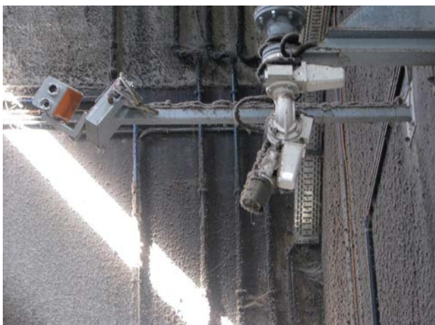
Figure 3: The PYROsmart® device works reliably even under permanent dust exposure. The apertures of the optics for IR and video are permanently flushed with a compressed air jet, which keeps them clean and clear.
