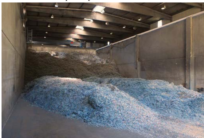
Figure 1: This type of RDF warehouse carries a high fire load and should therefore be especially protected against fire outbreaks.
