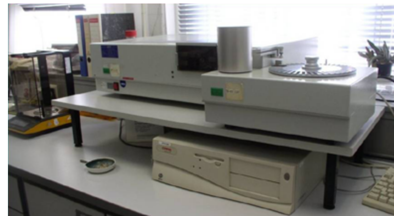
Figure 3: Example of a mercury analyser based on AAS. (Source: F. Wanzura, CEMEX Ostzement GmbH).
