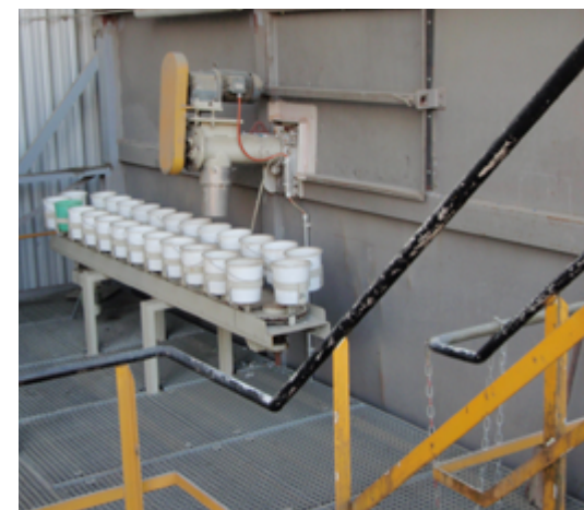
Figure 1: Fully automatic sampling at RDF unloading station. Left: Sampler. Right: Sample buckets.
