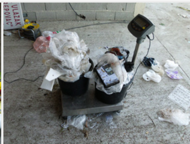
Figure 13: Buckets filled with plastics on a platform scale.
