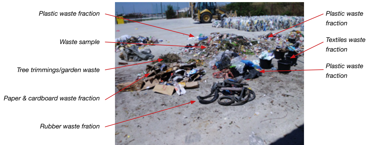
Figure 8: Typical arrangement of manually sorted waste components around the waste sample.
