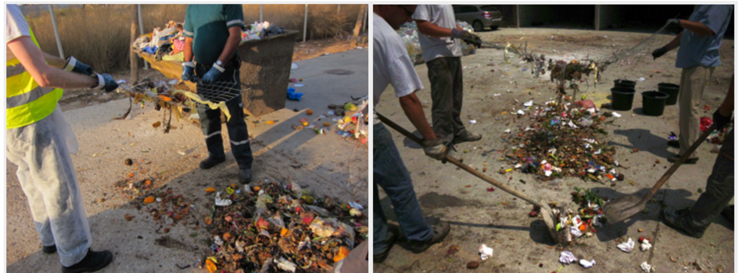
Figure 10: Sieving of the residues from handpicking: Sieve retention 5.5 cm, mostly consisting of fruit, and leftovers.
