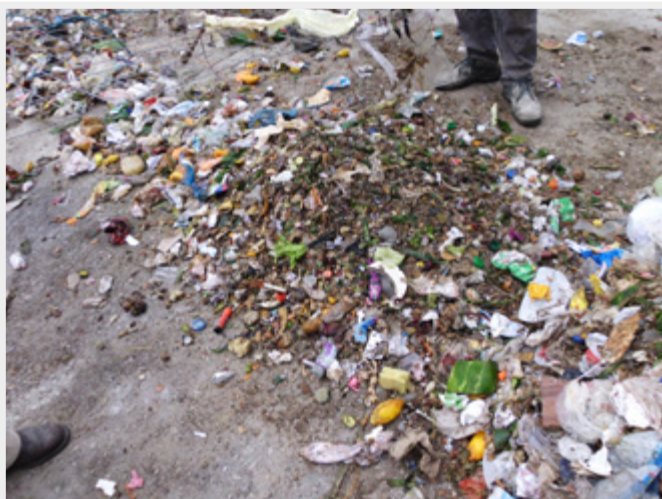
Figure 11: Passing 5.5 cm: Mainly organics, soil and small plastic and paper particles.
