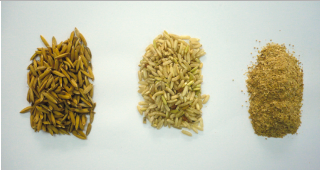
Figure 1: From rice husk to powder (Source: APAC Commodities Pte Ltd, Singapore).
