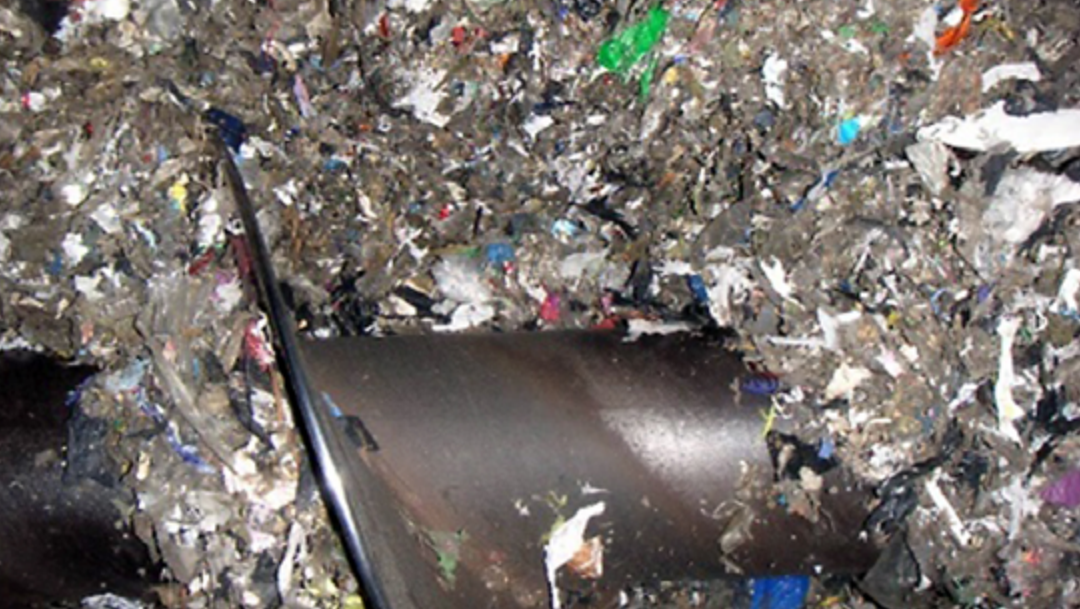
Figure 1: SRF in a screw conveyor
